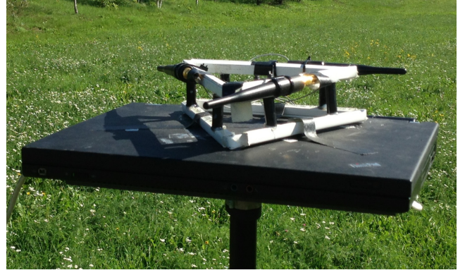
Figure 4: Base station with triangular antenna setup.
