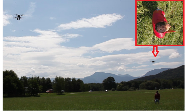
Figure 5: UAV detects the person by the red color of the jacket.
