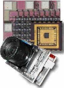
Integration of photo detecting elements and processing circuits on the same chip, to obtain better performance from sensors
