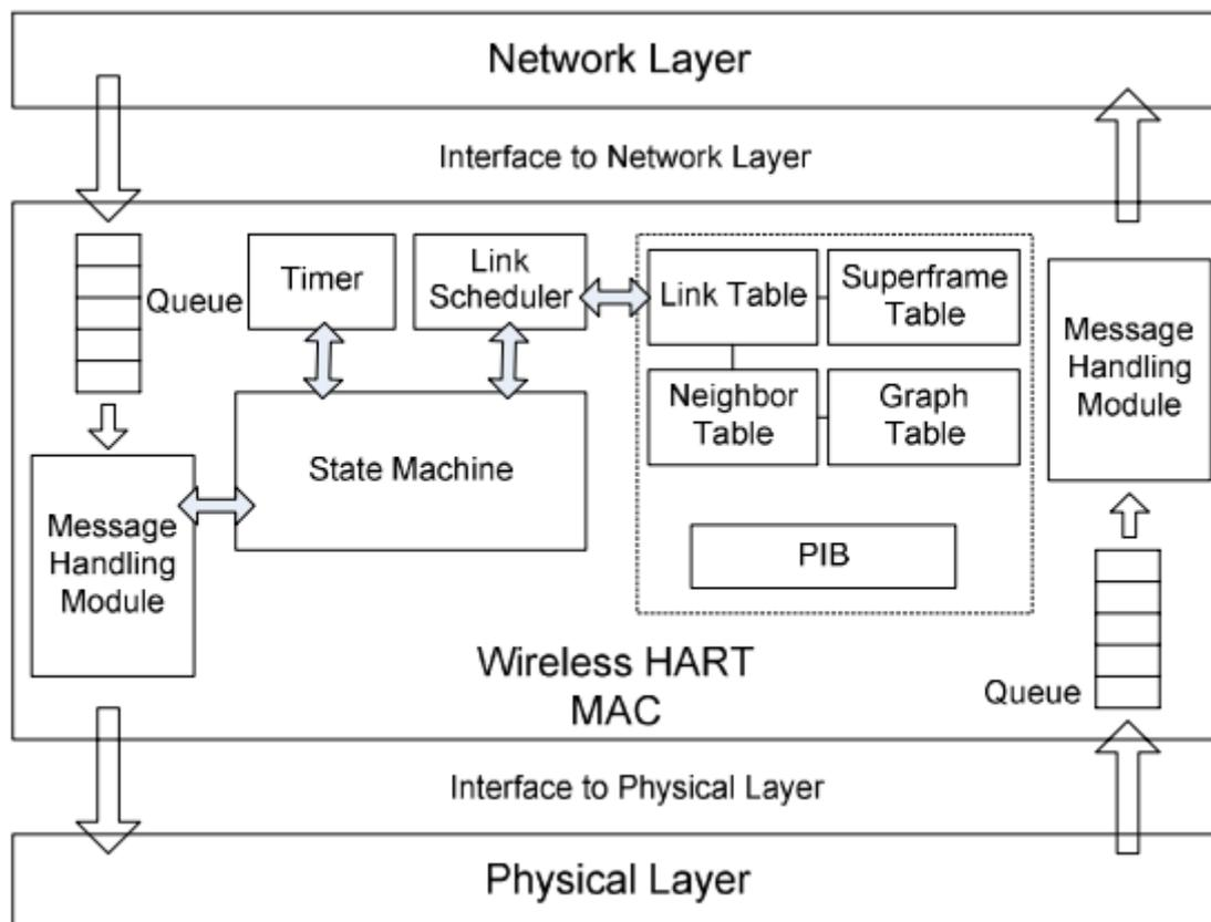
Figure 2 WirelessHART Data Link Layer Architecture [1].
