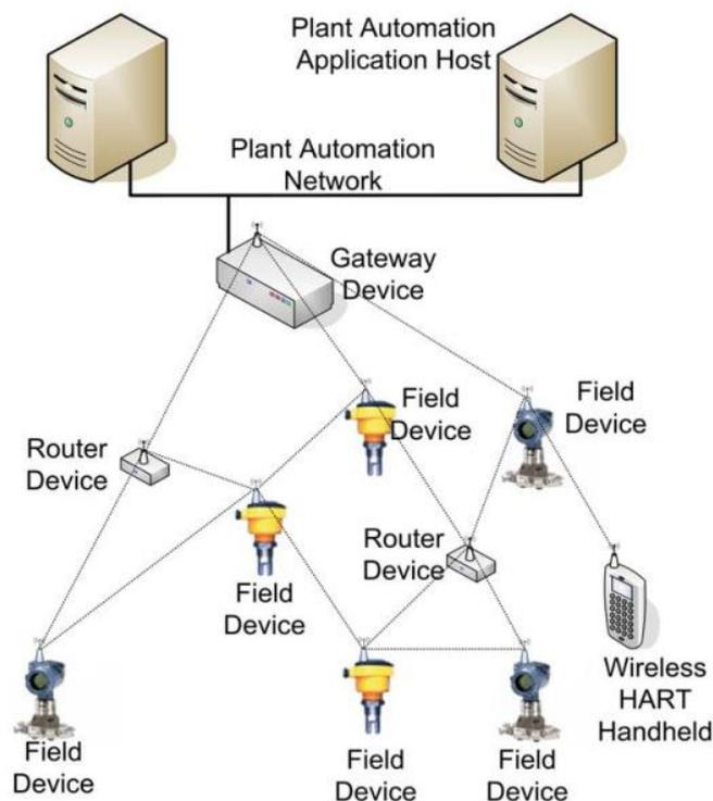
Figure 1 WirelessHART Mesh Networking
