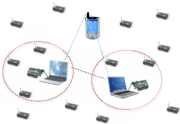
Figure 2. Operational scenario showing one hop communication between base stations (laptops) and motes and multi-hop communication among base stations and clients (PDAs). Client agents can also be co-located with the base stations (e.g., running on the laptops).
