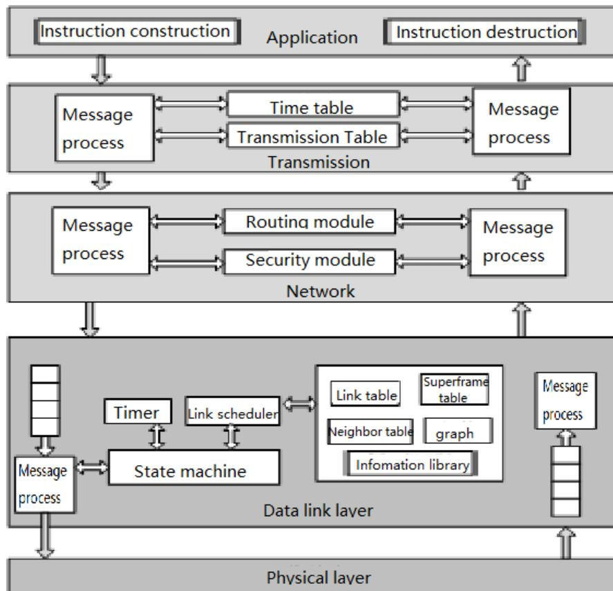
Figure 3-1: Overall Architecture of WirelessHART [3]
