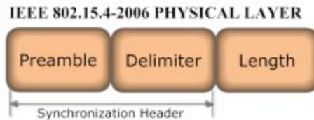
*Figure 3. WirelessHART Physical PDU Structure [6]*
