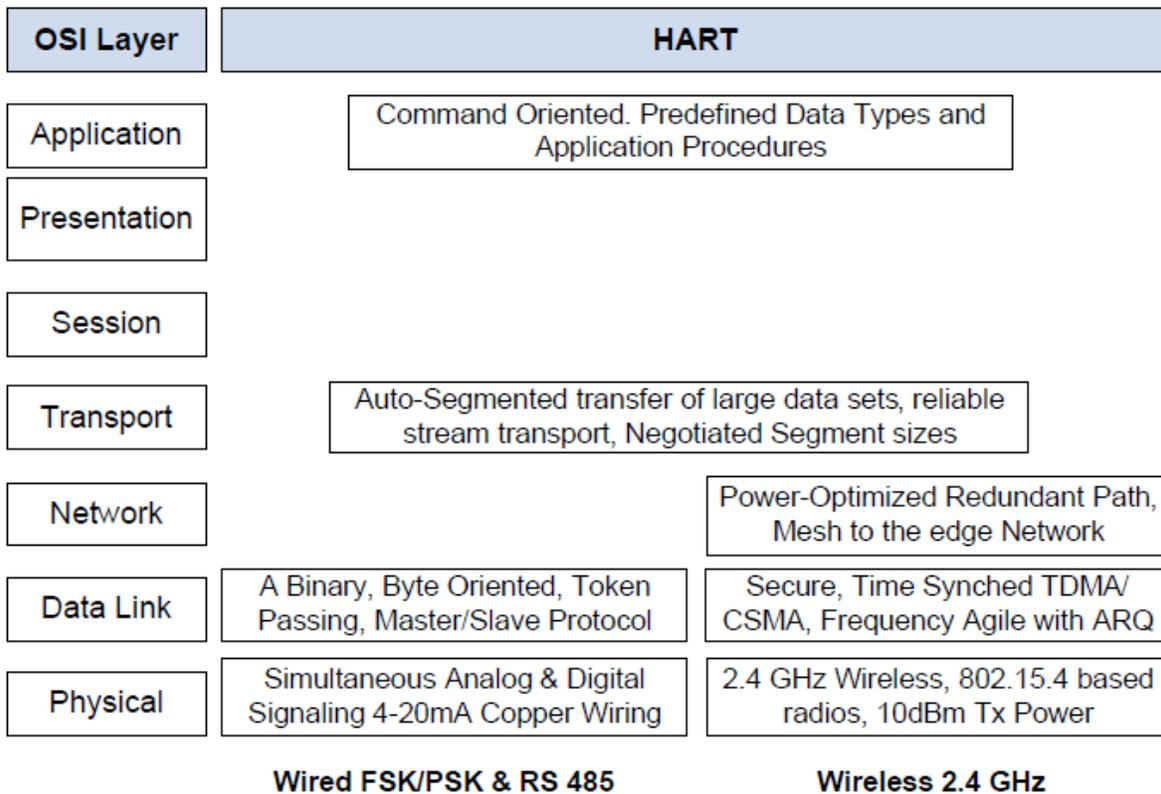
Figure 2. Architecture of HART Communication Protocol [1]
