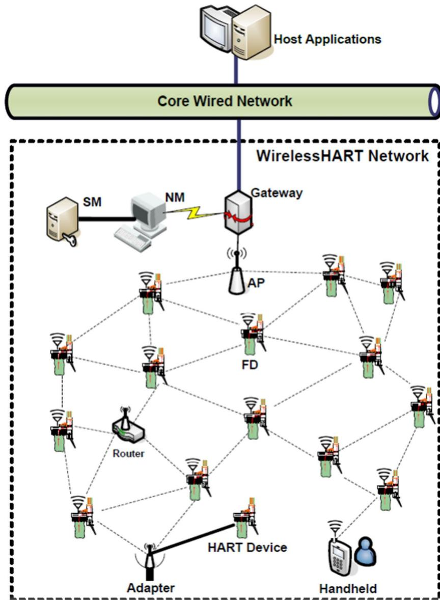
Figure 1. WirelessHART Network Components[4]
