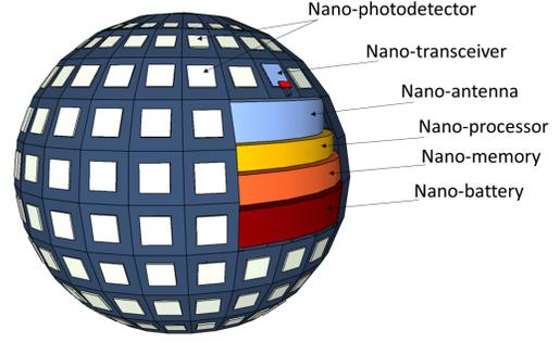
**Figure 3: Spherical constellation of a nano-camera resulting in a fully omni-directional sensor. The electrical components including nano-battery, -processor, -memory and -transceiver are placed within the sphere.**
