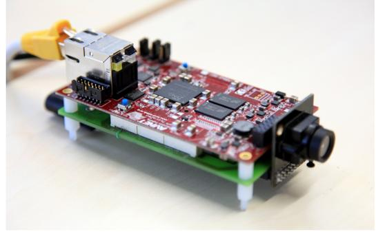
Fig. 3. Zynq7010 SoC and OV5642 image sensor based smart camera: It ensures video data integrity, authenticity, confidentiality and freshness using camera fingerprint extracted from hardware using on-chip PUF
