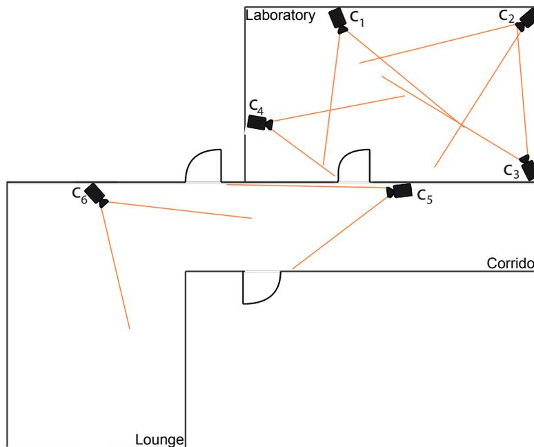
**Fig. 13.3** The smart camera network composed of six cameras deployed in an indoor environment. The cameras are depicted by a black camera symbol and their FOVs are indicated by orange lines.
