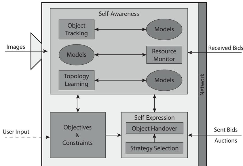
**Fig. 13.1** The architecture of a self-aware and self-expressive camera node composed by six building blocks
