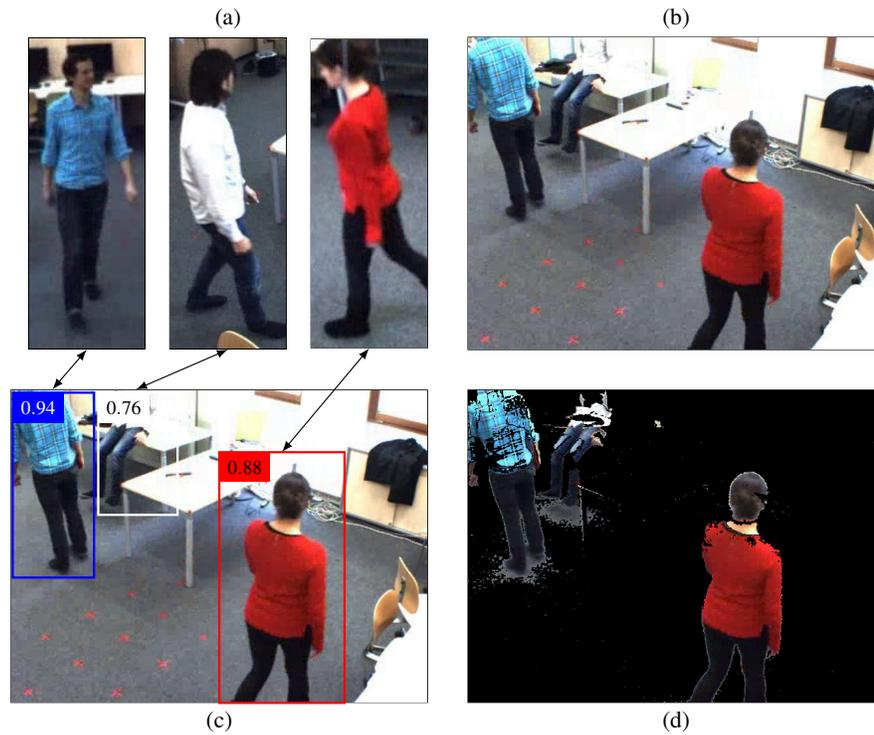
**Fig. 13.2** Object tracking approach. (a) Template database images, (b) original image, (c) matching results between foreground objects and objects templates, (d) foreground image
