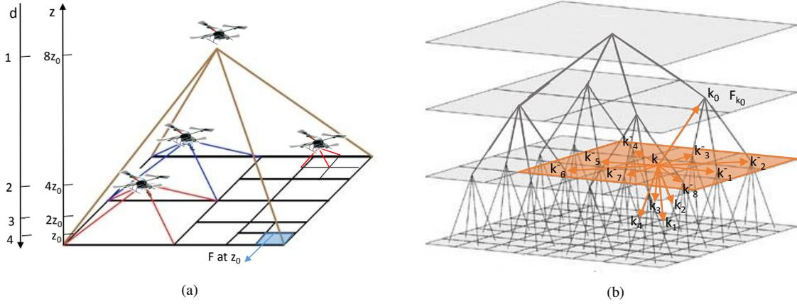
Fig. 2: Model for the MAV movement: (a) Relationship of search region  $\Omega$ , FOV ( $F$ ), altitude ( $z$ ), lowest altitude ( $z_0$ ), and depth ( $d$ ) of the quad-tree. (b) Fourteen-neighborhood (orange arrows and square around the current node  $k$ ).
