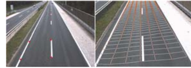
Figure 2. Calibration points (left) and 1-by-1 meter grid, computed from obtained camera parameters (right)
