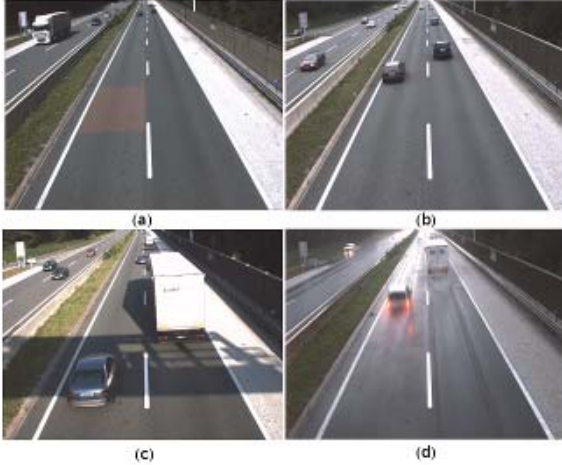
Figure 7. (a) Region of interest used for evaluation, (b) dry road with small shadows, (c) large shadows, (d) water on the road
