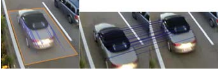
Figure 3. Vehicle in ROI with KLT motion vectors (left) and KLT feature matching (right)
