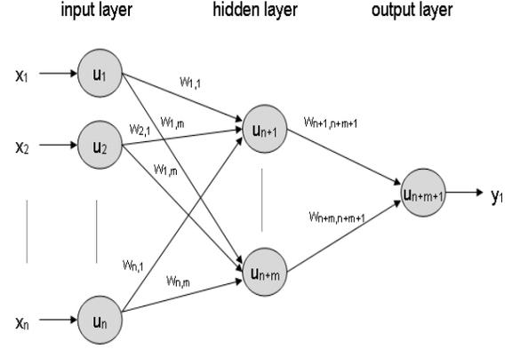
Figure 4: A three-layered feed-forward ANN representing a  $FFU_i$  with respect to cluster  $c$
