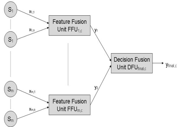
Figure 2: Feature and decision fusion with reference to fusion cluster  $c$  (PFC), where  $S_i$  represents sensor node  $i$ ,  $x_{i,j}$  the  $j^{th}$  feature value of sensor  $i$  and  $y_i$  the  $i^{th}$  local partial decision generated by  $FFU_{i,c}$ .
