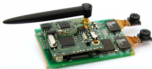
Figure 1. WiCa: Wireless Smart Camera.
