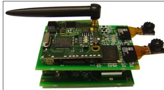
Figure 1: WICA camera (6x4x3cm) shown with 2 VGA sensors
