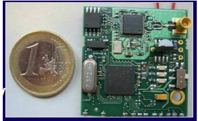
Fig. 9. The ZigBee transceiver module used on the camera.
